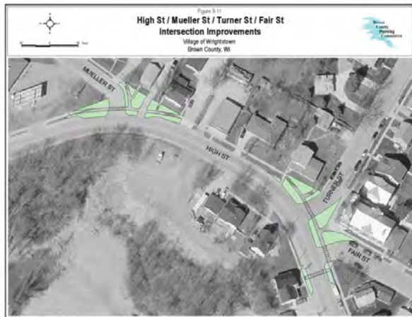
Figure 3-11: High St/Mueller St/Turner St/Fair St Intersection Improvements
