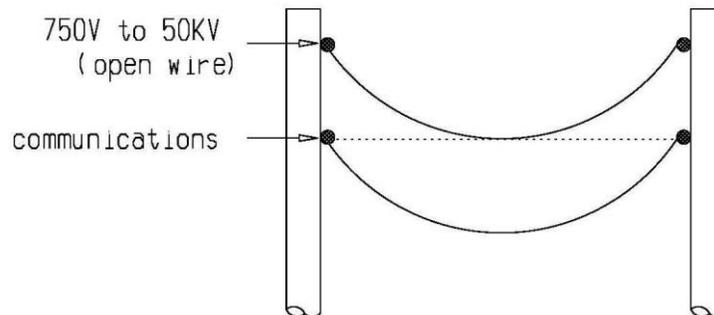
For power service drops running above and parallel to communication service drops, 12 inches of clearance is required in the span between *covered* power services and communication services (NESC 235C Exception 3). 40 inches of clearance is still required at the pole.
