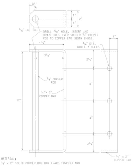
$^{1}4^{\prime\prime}$  imes 2" SOLID COPPER BUS BAR (HARD TEMPER) AND 3/4" DIANETER SOLID COPPER ROD (HARD TEMPER).
